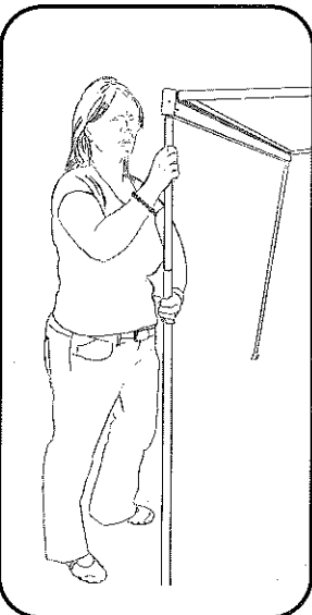
Extend legs to height required and twist to lock in place. NB. Should it rain, drop one leg in order for water to run off EEZI-AWN.
