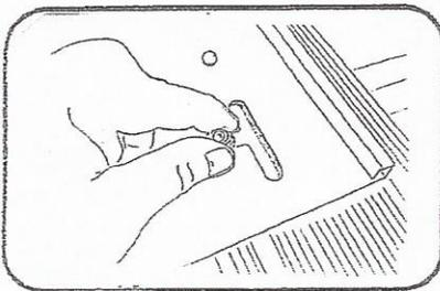
Thread nylock nuts onto bolts positioned.
