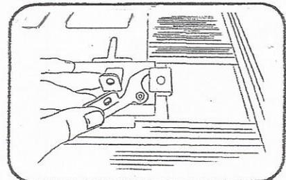
Slide lock plate closed and lock Alubox onto tray.
