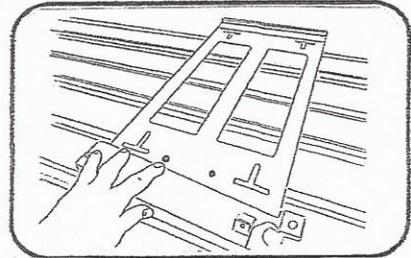
Place k9 Alubox tray onto rack in required position
