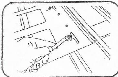
Tighten with 13mm spanner wrench.
